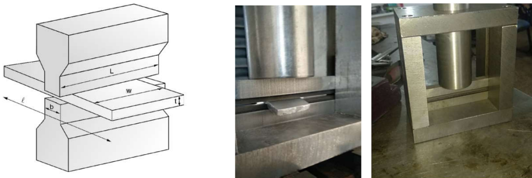
Fig. 1. An apparatus made for plane strain compression test.
