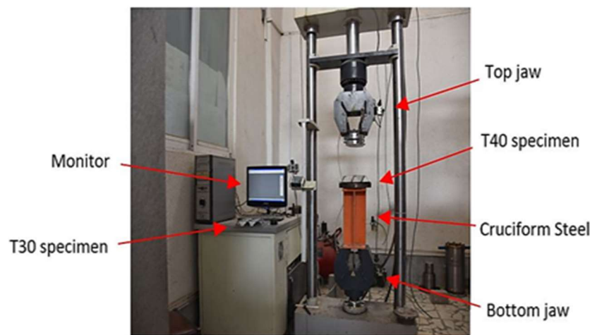
Fig. 4. Santam STD-600 compression testing machine
