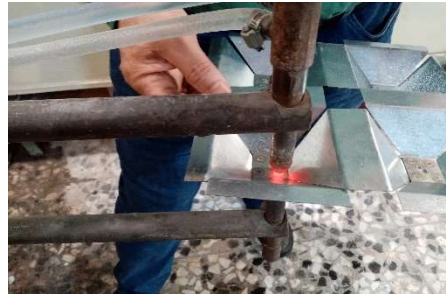
Fig. 3. Spot welding the basic compartments of the core
