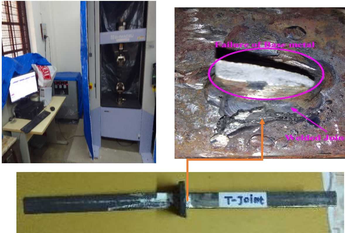
Fig.4. Experimental analysis by using UTM machine
